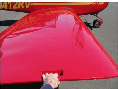
Tie-Down – UNTIE the tie-down rope/chain, REMOVE eye bolt if desired.
