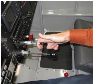
Fuel shut-off valve is used to permit or prevent fuel from flowing to the engine compartment. It may be pulled up to the 'OFF' position to prevent fuel flow, or pushed down to the 'ON' position.
