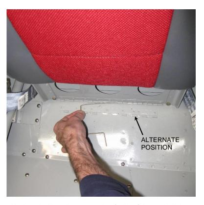
Additionally the seatback recline angle can be adjusted by how the hinged spacer on the aft side of the seatback is positioned. The seatback position and recline angle can be adjusted independently of each other.
