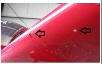
Wing Hand Hold - APPLY FORCE fore/aft & up/down; CHECK no free movement
