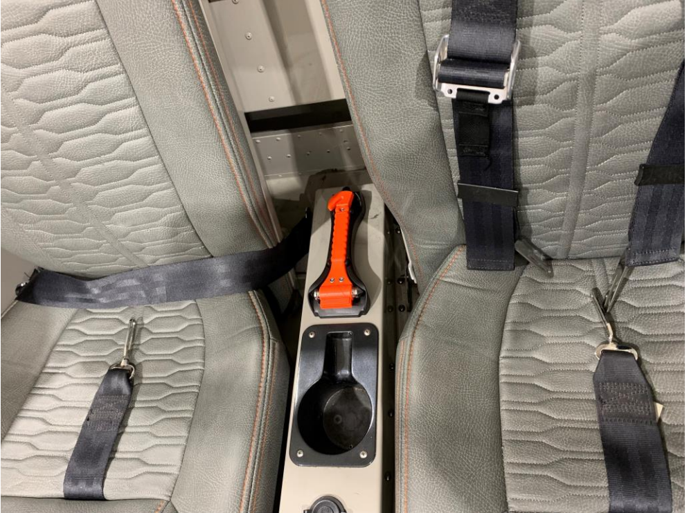
FIGURE 7-13 EXAMPLE EGRESS HAMMER LOCATION
