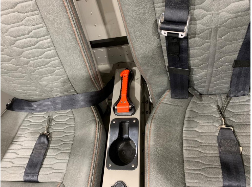
FIGURE 7-13 EXAMPLE EGRESS HAMMER LOCATION
